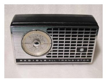
It did not have a telescopic antenna, so to improve reception I fitted one with a wire loop around the internal ferrite rod. Reception was improved further when I fitted a socket to the radio and
